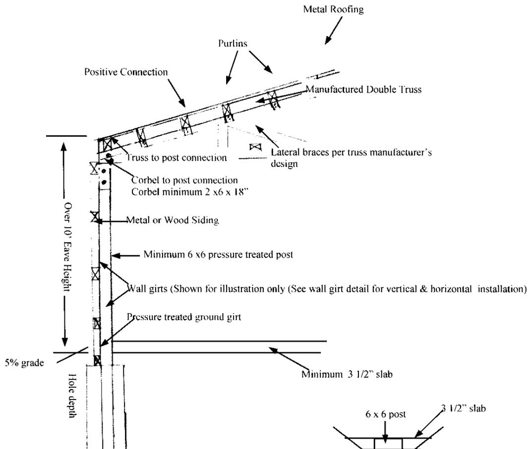
3'6" hole depth with hairpin anchor to concrete or 48" depth if a slab is not being installed.
